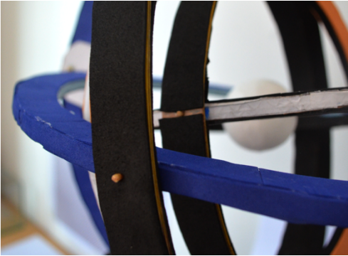
FIG. 6. Fastening Ch to Ch using a piece of wood stick as a “rivet” at the West cardinal point. The hour angle circle ( Ch ) can be adjusted to the observer’s latitude.
