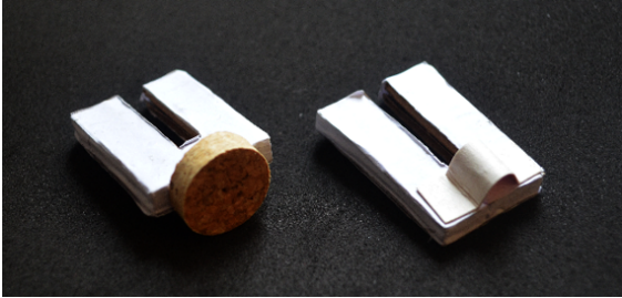
FIG. 5. Finished bearings of the celestial axis ( Fp ). The measures of each piece follow the diagrams of Fig. 12.
