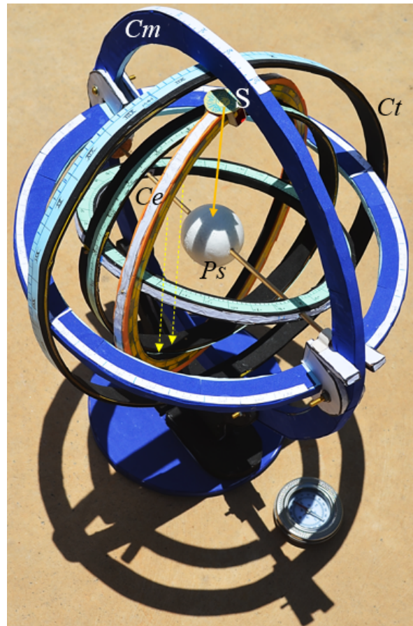
FIG. 10. The armillary sphere as a sundial. The sun S casts a shadow on Ps on March 4 2023 at 12:23 local civil time corresponding to 12:00 of the local true solar time at the observer coordinate (longitude 48.01^\circ W ). A magnetic compass was used to find the meridian line. The shadow of Ce is also exactly on Ce which occurs for the sun's longitude for the date.
